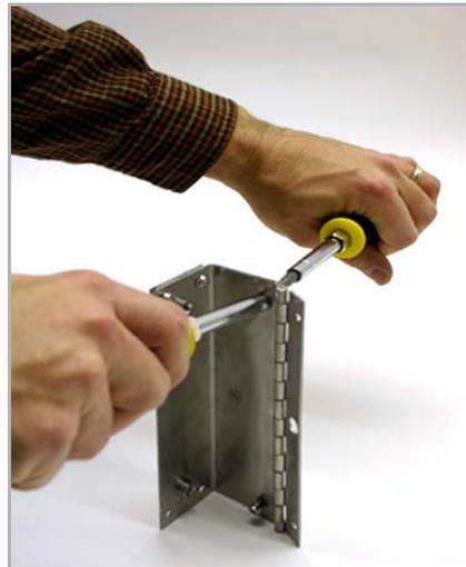
*Figure 2-8 Assemble the hinges and brackets*
