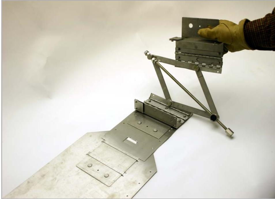
*Figure 2-14 Scissors mechanism connected with extension and base*
