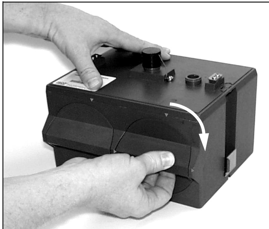
Figure 1-15 Battery Module - closing the door
