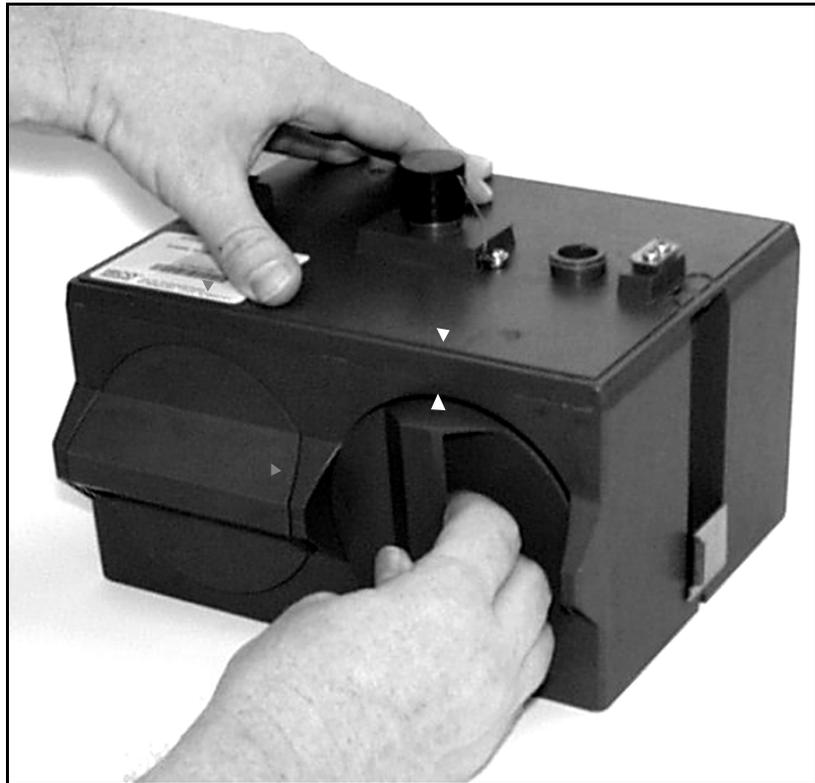
Figure 1-14 Battery Module - aligning the door
