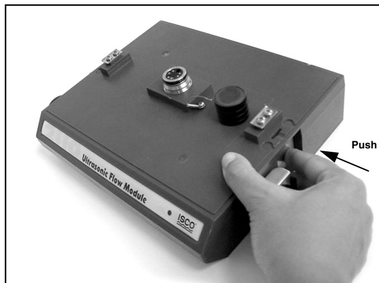
Figure 1-5 Unlocking the latch
