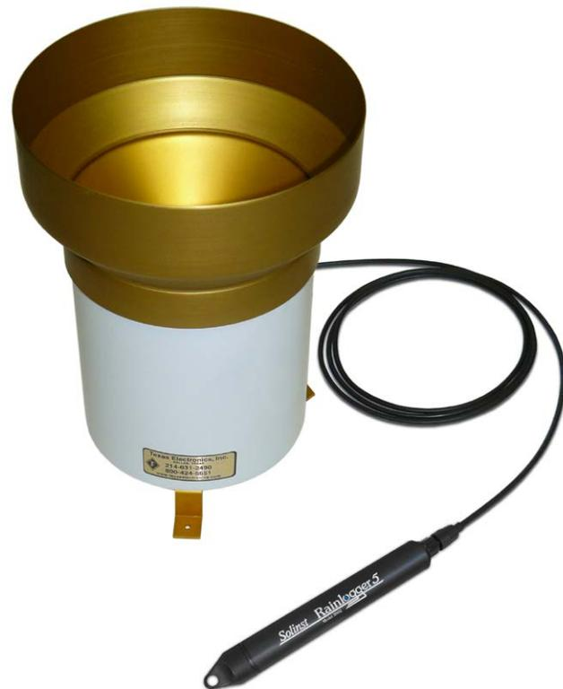
Figure 10-21 Rainlogger 5 Connected to Tipping-bucket
