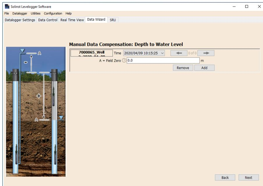
Figure 8-9 Manual Data Adjustment - Depth to Water Level
