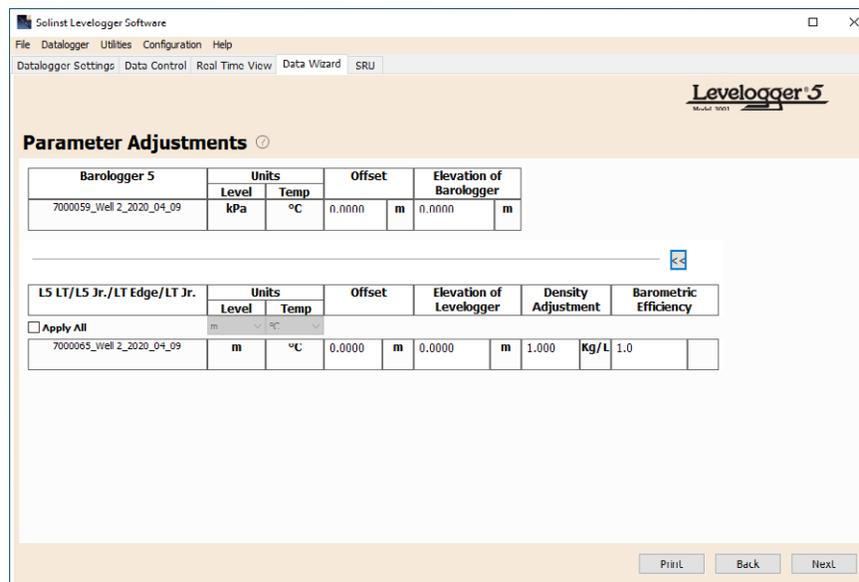
Figure 8-8 Parameter Adjustments
