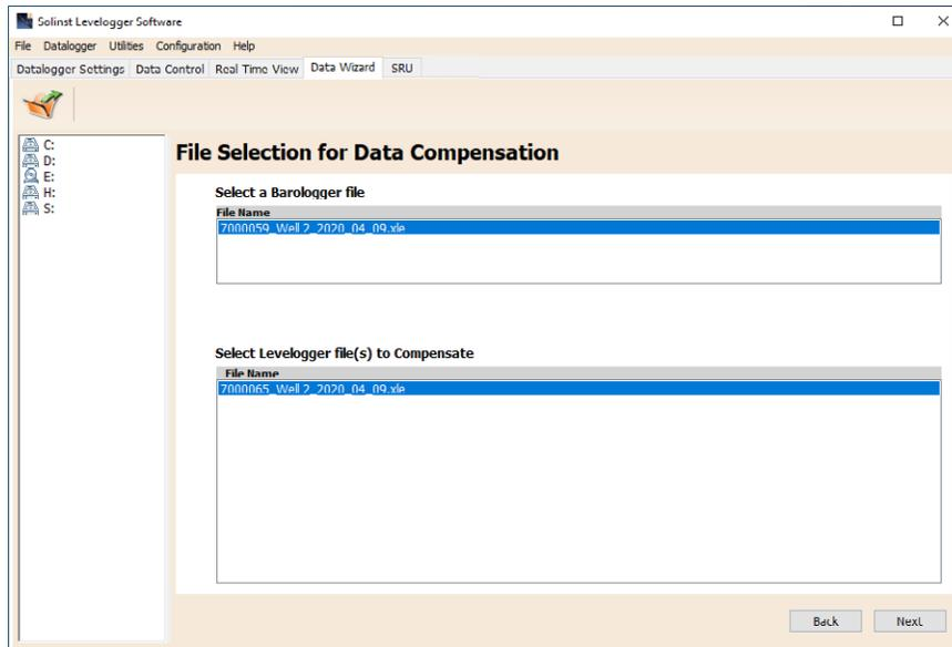
Figure 8-7 Selecting Files for Compensation
