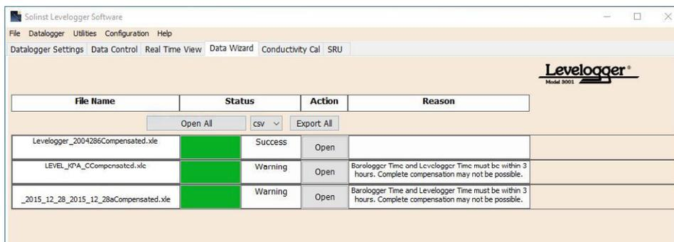
Figure 8-4 Barometric Compensation Results - Multiple Files
