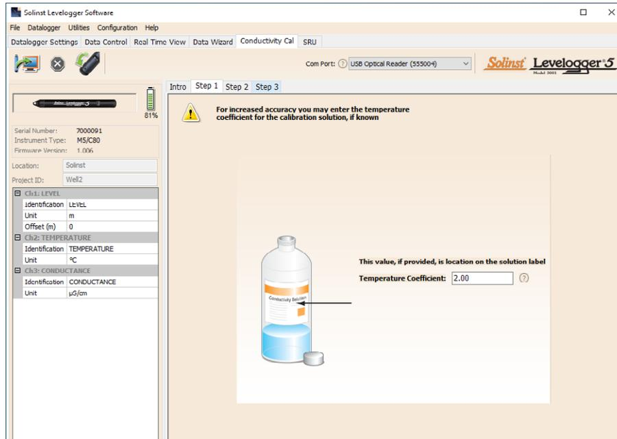
Figure 6-3 Levellogger Conductivity Calibration Wizard Step 1
