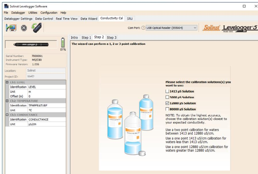
Figure 6-4 Levellogger Conductivity Calibration Wizard Step 2
