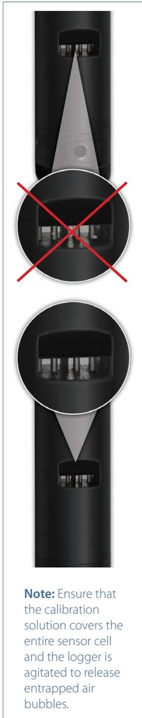
**Note:** Ensure that the calibration solution covers the entire sensor cell and the logger is agitated to release entrapped air bubbles.
