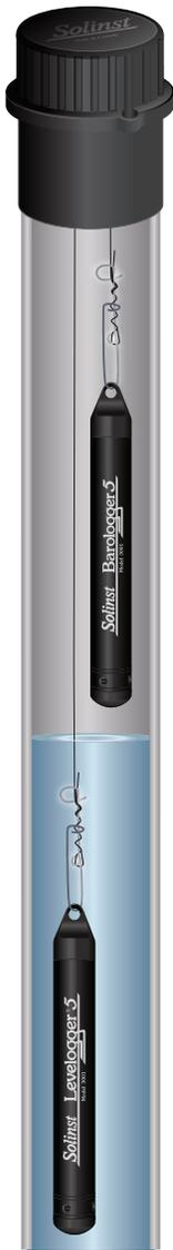
Figure 10-18 Levellogger and Barologger in Well
