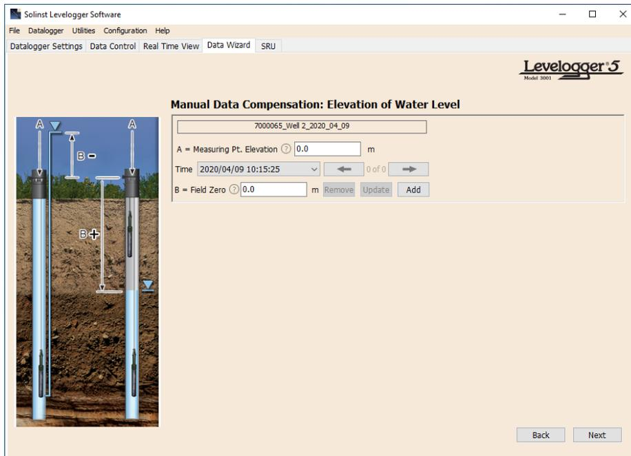
Figure 8-10 Manual Data Adjustment - Elevation of Water Level
