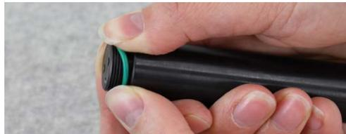
Figure 10-26 Replacing Levellogger O-rings
