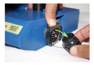
Figure 2-8 Preparing the 2160 connector receptacle
