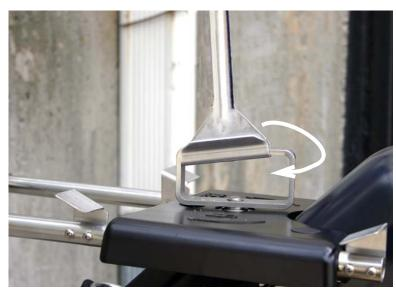
Figure 2-20 Turn the locking handle clockwise until sensor is locked into place (shown with sensor retrieval arm, described in Section 2.7)
