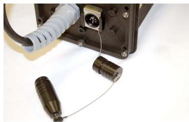
4. Aligning the pins on the Laser-Flow cable with those in the connector receptacle, push the 350 connector into the receptacle on the inner wall of the LaserFlow until the spring release clicks.
