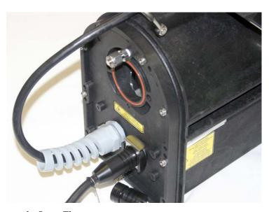
Figure 5-14 Connecting the 350 AV sensor to the LaserFlow
