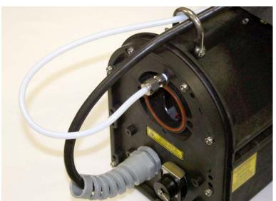
Figure 5-7 Attach gas tubing to inlet
