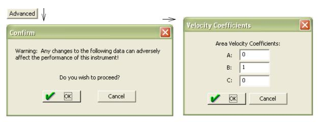
Figure 4-11 350 Velocity tab: Advanced settings for optional TIENet 350 AV sensor
