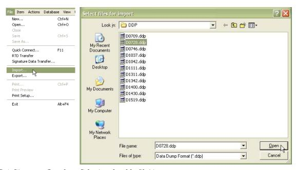
Figure B-1 Signature flow data: Selecting the .ddp file(s)
