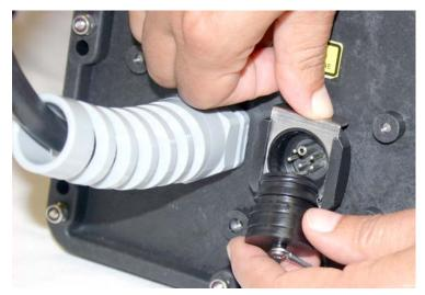
3. Remove the cap from the 350 TIENet plug and push the protective caps of the two sensors together.
