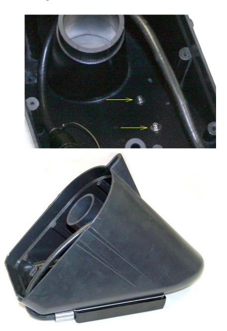
Figure 5-13 Mounting the integrated 350 AV sensor on the LaserFlow
