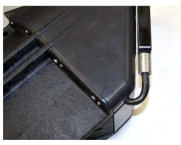
Figure 5-15 Reassembling the LaserFlow w / AV sensor installed
