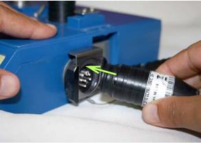
Figure 2-9 Secure caps and connect LaserFlow to 2160
