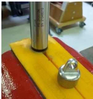
*Cableless Sensor—gripping on knurled area*
