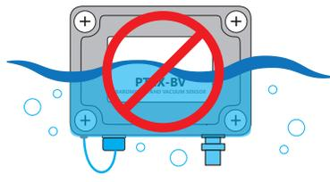
**Don't install so box or connector is submerged**
