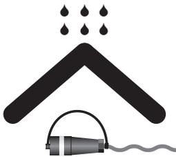
**Do install sensor so the connector end is kept dry**
