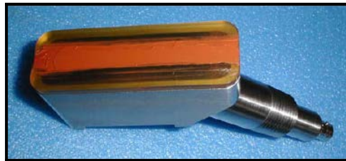
Figure 25: Couplant on Transducer Face
