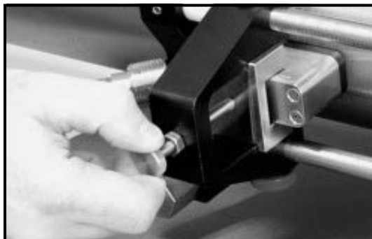
Figure 26: Installing the First Transducer
