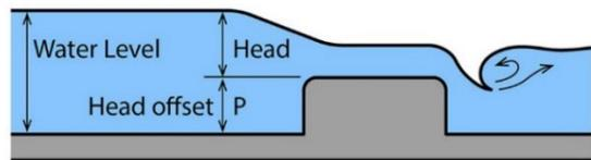
For other types of flumes, such as this example diagram where the water level (or H) is being measured from the bottom of the flume:
