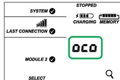
If a water level sensor module is installed, the channel count is listed as 4. This represents barometric pressure, water pressure, differential pressure, and water temperature. Water level and water flow channels are derived in HOBOLink and not included in the channel count shown on the station LCD.
