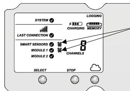
Tripped smart sensor alarm and analog sensor alarm
