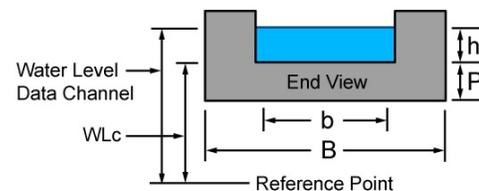
The HOBOLink water flow calculations for a rectangular weir assume the following:
