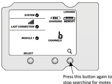
Measurements will be recorded at the logging interval specified in HOBOLink, transmitted to the RX3000 station, and uploaded to HOBOLink at the next connection interval (readout).
