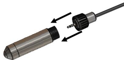
**Important:** Make sure the O-rings on the cable jack end and the sensor mating housing surfaces are clear of any debris. Any contamination of these surfaces can cause leaks that may lead to sensor failure.
