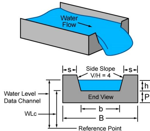
The HOBOLink water flow calculations for a trapezoidal weir assume the following:
