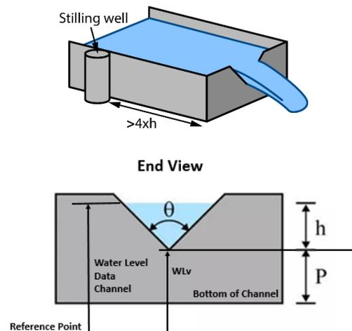
The HOBOLink water flow calculations for a v-notch weir assume the following:
