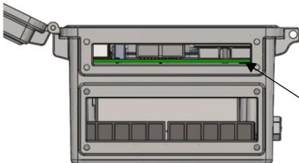
Feed analog sensor, relay, and water level sensor cables through this opening to connect them to the optional modules
