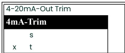
Press the [▲] and [▼] key until your output device reads exactly 4 mA. When done, press **[ENTER]**.
