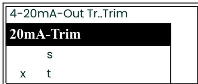
Press the [▲] and [▼] key until your output device reads exactly 20 mA. When done, press **[ENTER]**.
