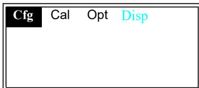
If necessary, use the [◀] and [▶] keys to select [Cfg] and press [ENTER]. (Notice *Disp* is unavailable at this time.)
