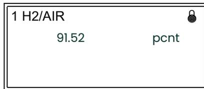
The meter returns directly to run mode, with the padlock icon indicating that the *User Program* is now locked.
