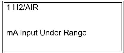
This message appears for a few seconds, until the sensor begins outputting a valid gas content signal.
