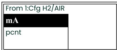
A list of available units is shown. Use the [▲] and [▼] keys to select the desired units and press [ENTER].
