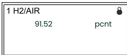
While in measurement mode, press the **[ESC]**, **[ENTER]**, and **[ESC]** keys in sequence.
